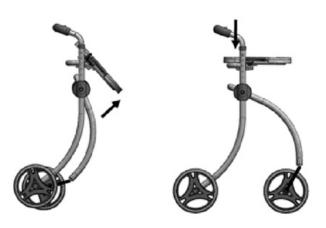
To ensure the rollator is fully open, support the handle with one hand and press on the tray with your other hand. When fully opened, you will hear a 'click' informing you the frame is locked in position.
