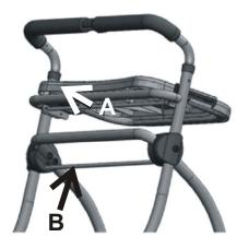
Grasp the tray folding bar and pull in the direction shown by arrow A. The tray will drop down.
