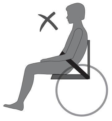
Incorrect placing of belt
