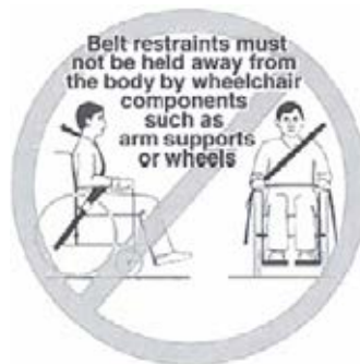
Improper Positioning of Belts on Occupant
