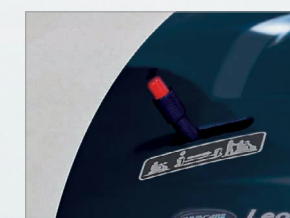
Two-step disengaging lever to prevent free-wheeling
