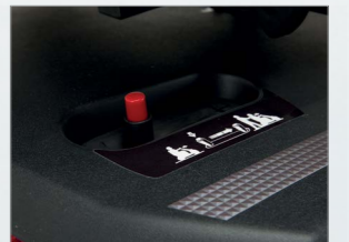
Two-step disengaging lever to help prevent free-wheeling
