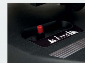
Two-step disengaging lever to help prevent free-wheeling
