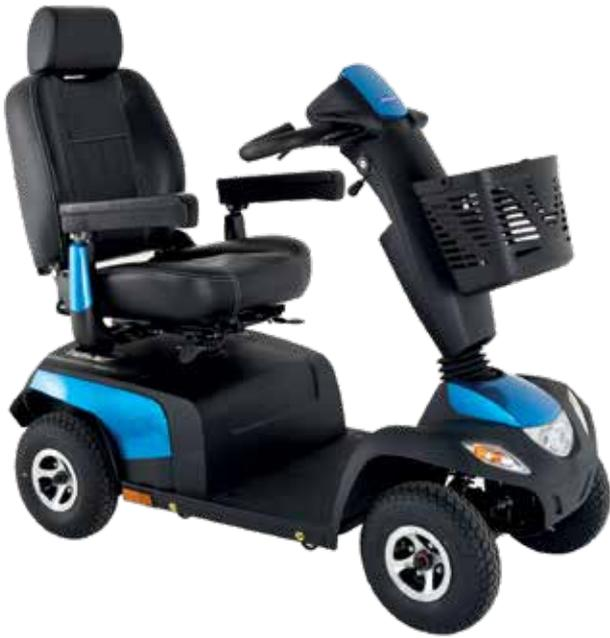
The advanced suspension system on the Pegagus PRO has been designed to bring better performance and give a smoother ride over a variety of surfaces and terrains. In addition, the Pegagus PRO features a powerful motor and 12" pneumatic tyres to ensure that whether you are in the city or the country, you get where you need to go in comfort and style.
