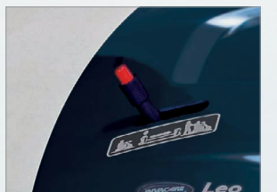
Two-step disengaging lever to prevent free-wheeling
