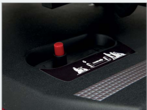
Two-step disengaging lever to help prevent free-wheeling
