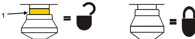
**Safety side operation knob shown in unlocked and locked**
