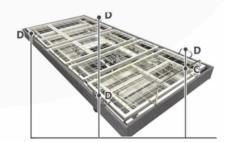
5. Cut off and discard the zip-tie lines securing the power supply, handset control, and moving parts of the frame. The locations of these are found in items 1-6 below.
