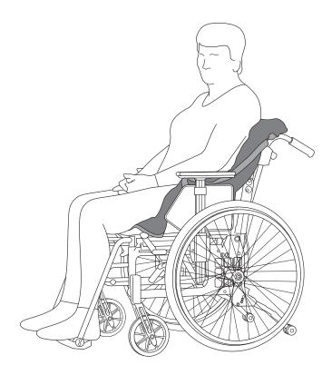
C5. The sling is supposed to remain under the user after transfer.
