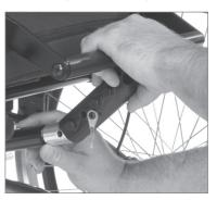
· Lock the backrest by pushing the locking bolt through the plastic bracket and gas spring locking head.
