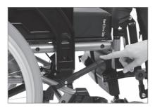
• To reposition the brake, loosen the two screws on the inside of the brake clamp.
