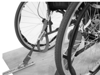
Fitting the rear restraint
