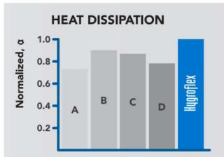
Thermal diffusivity (α) measures the rate of heat transfer of a material from the hot side to the cold side. In a substance with high thermal diffusivity, heat transfers rapidly through it.
