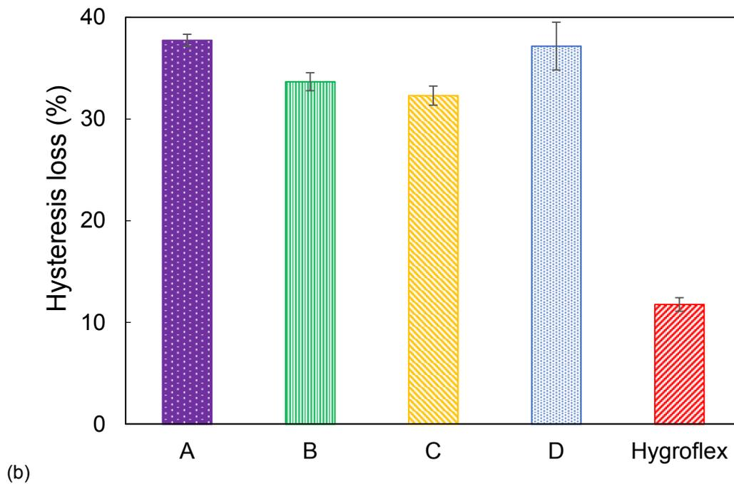
Figure 2-20: (a) Energy dissipated and (b) hysteresis loss calculated from force-displacement curves for all foams.
