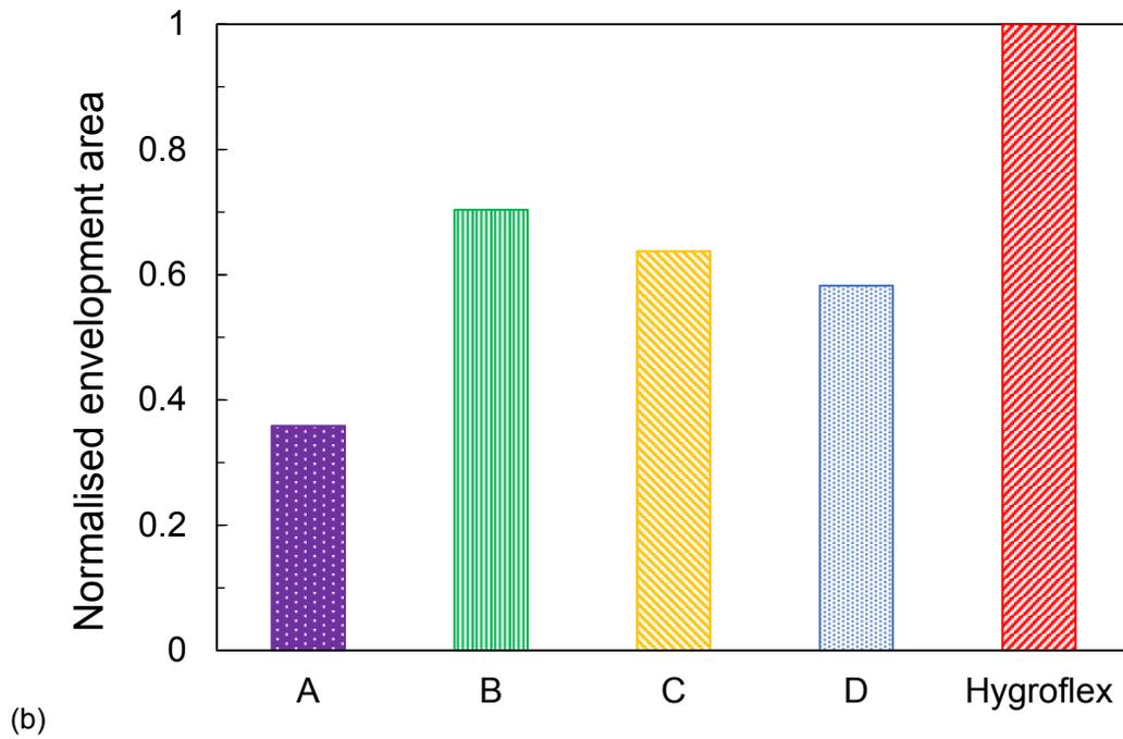
Figure 2-9: Normalised envelopment area for all foams under (a) 50 N and (b) 75 N loads (all samples were normalised against Hygroflex).
