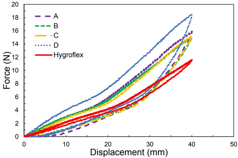
Figure 2-19: Representative force-displacement curves for all foams under cyclic loading.
