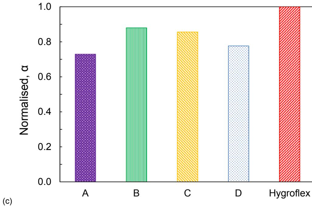
Figure 2-21: Normalised (a) specific heat capacity (c), (b) thermal conductivity (k) and (c) thermal diffusivity ( $\alpha$ ) for all foam materials.
