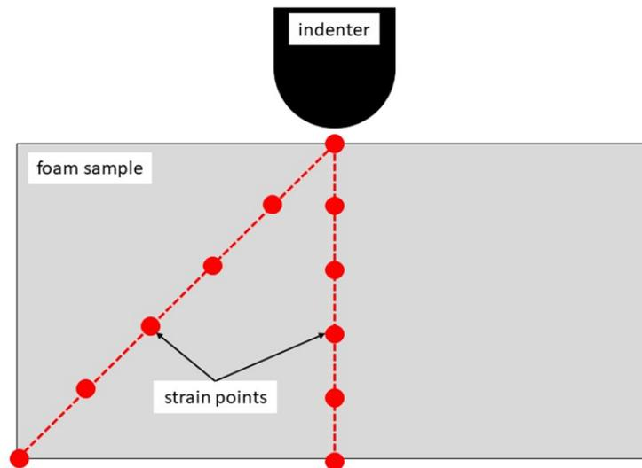
Figure 2-2: Schematic showing strain vectors through the thickness of foam.
