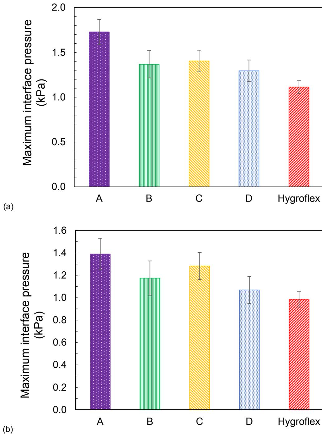
Figure 2-12: Maximum interface pressure (IP) (a) over entirety of test and (b) after two-minute hold for 40 % strain displacement control.
