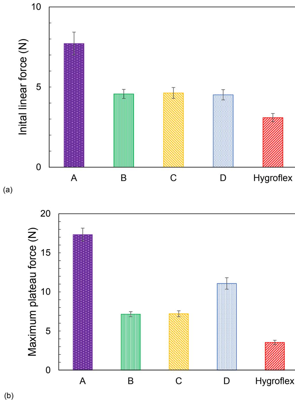
Figure 2-18: Roller-arm test force measurements; (a) linear force due to initiation of movement of the roller and (b) maximum plateau force after the roller completes one full rotation.
