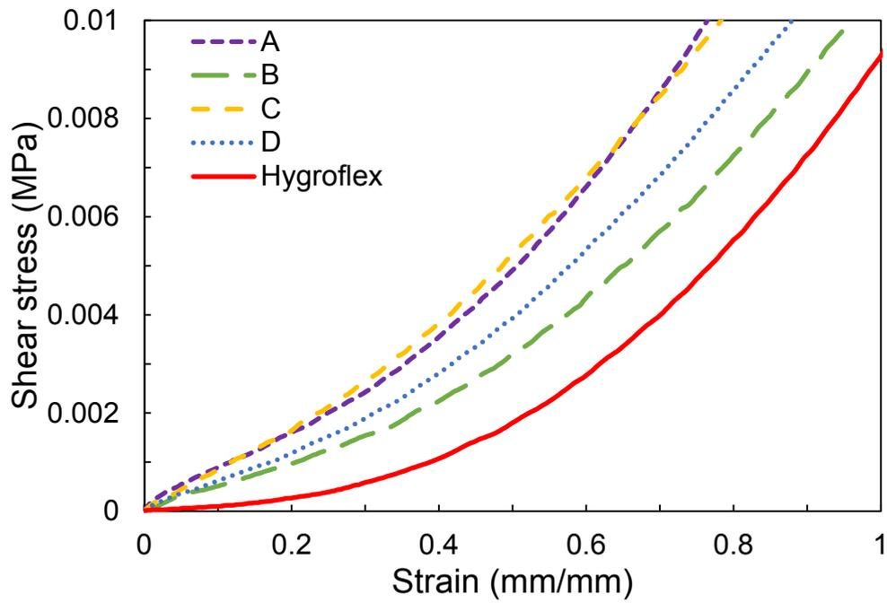
Figure 2-14: Representative shear stress-strain data for all foams.
