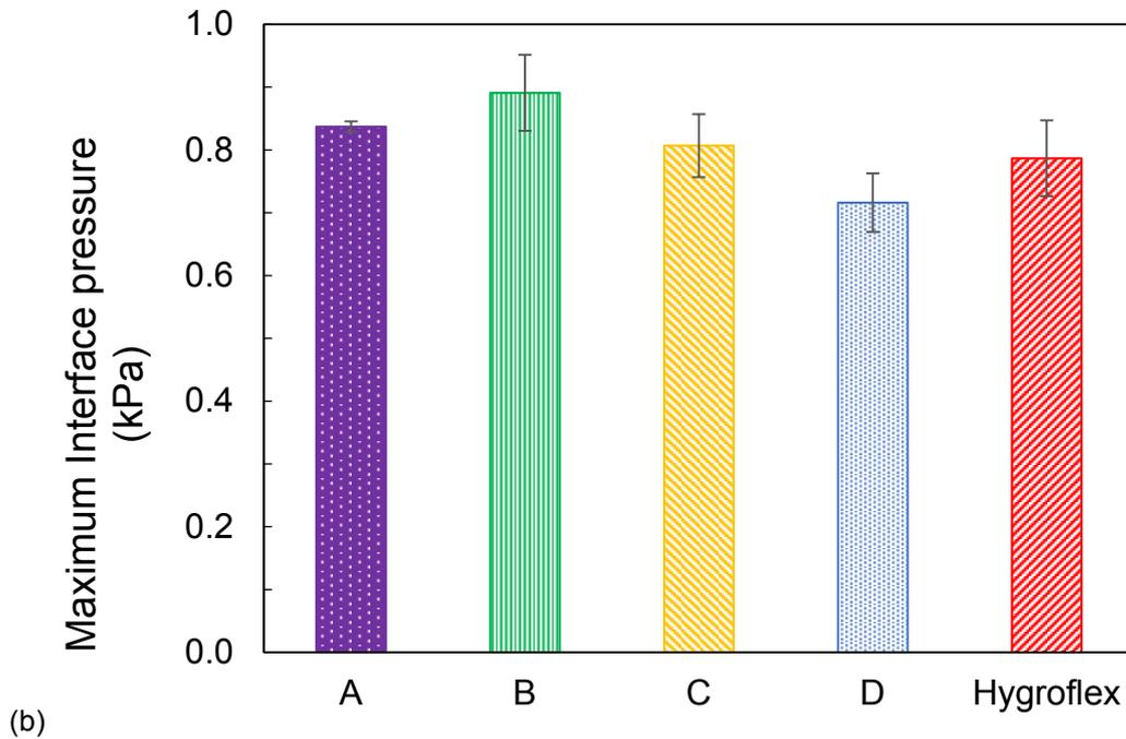
Figure 2-11: Maximum interface pressure (IP) (a) over entirety of test and (b) after two-minute hold for 75 N force control.
