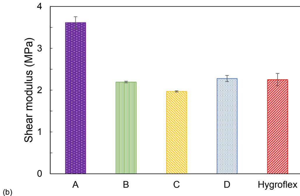
Figure 2-15: Comparison of shear moduli of all foams for (a) initial slope (0.1-0.3 % strain) and (b) post densification (1.0-1.5 % strain).
