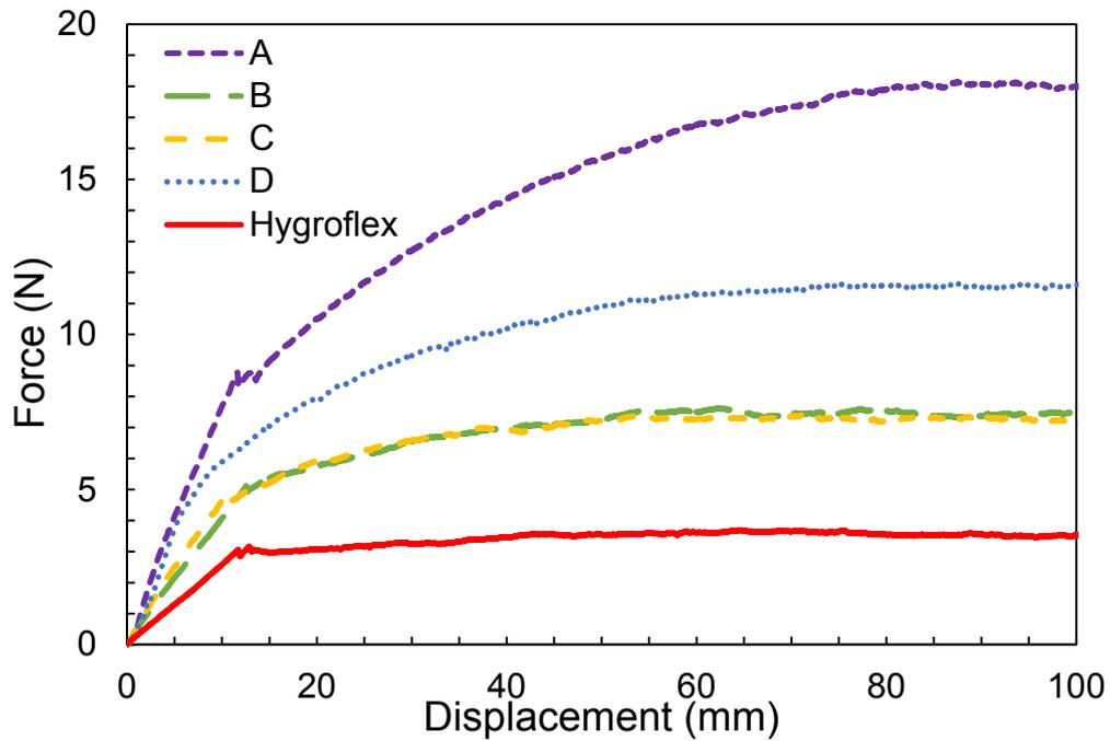
Figure 2-17: Roller-arm test force-displacement curves for all foams.
