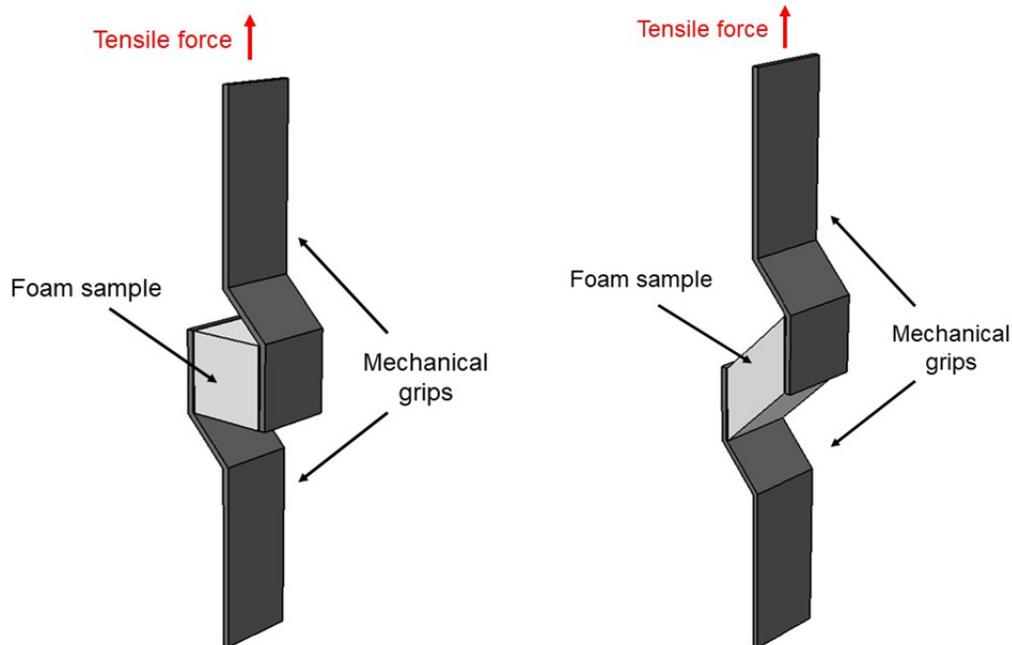
Figure 2-13: Schematic of the shear test with starting position (left) and final position (right).
