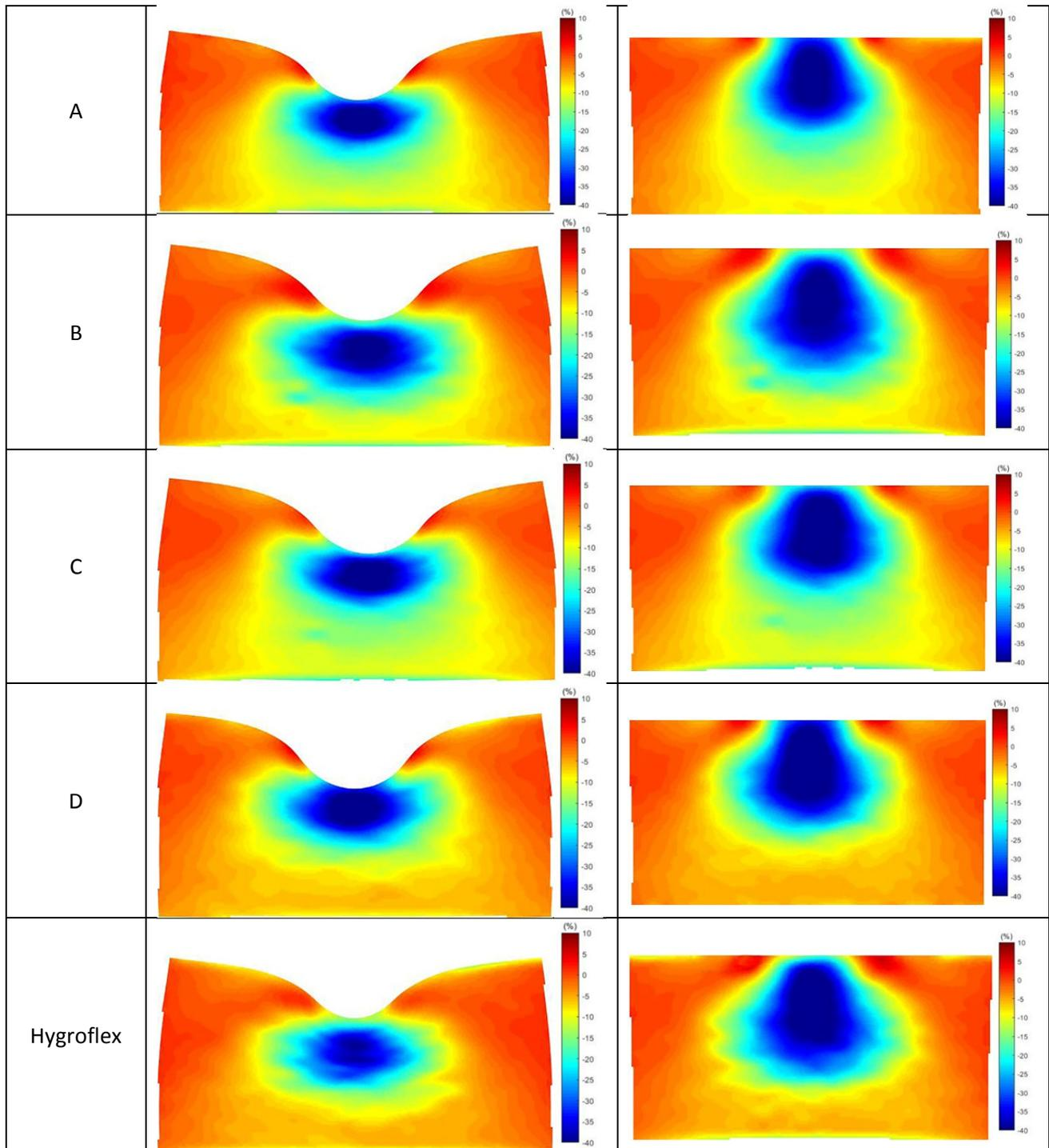
The strain field depicted in Table 2 represents the finite longitudinal strain ( $\epsilon_{yy}$ ) of each foam under 40 % compression from the sharp indenter. Figure 2-6 qualitatively highlights the fractional area of high-strain (15-40 %) in the foam. When compressed by 40 % of its initial thickness, the
