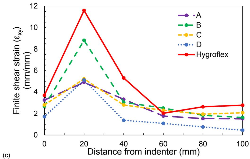
Figure 2-4: Force control (a) longitudinal (b) transverse and (c) shear strain values measured from directly under the indenter to the bottom left corner of the sample (angled line in Table 1).
