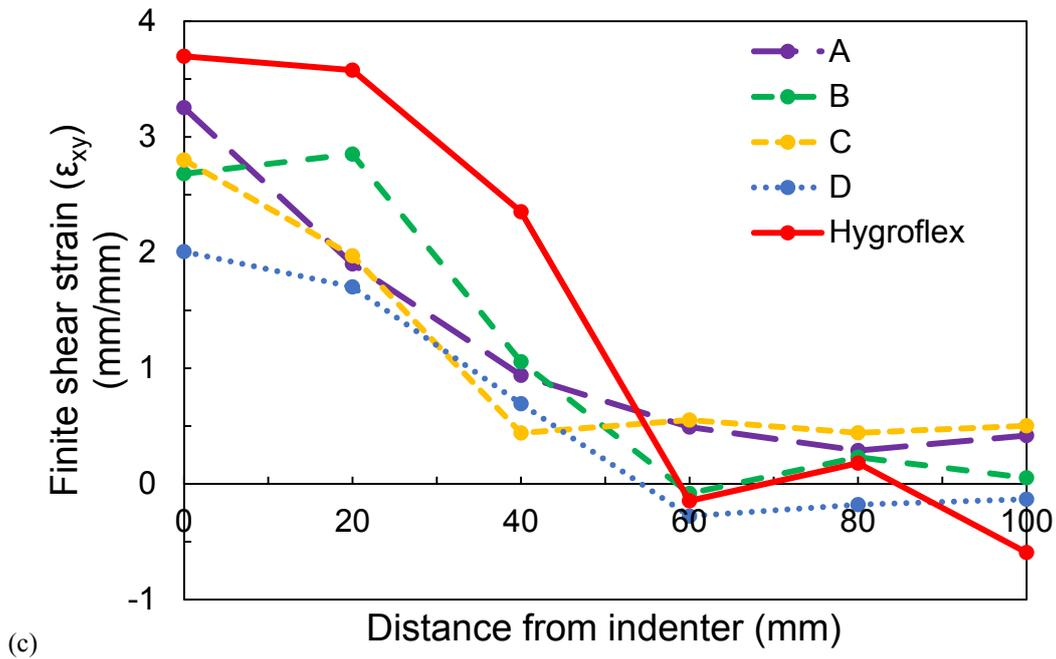
Figure 2-5: Force control (a) Longitudinal (b) transverse and (c) shear strain values measured from directly under the indenter to the bottom of the sample directly under the indenter (straight line in Table 1).
