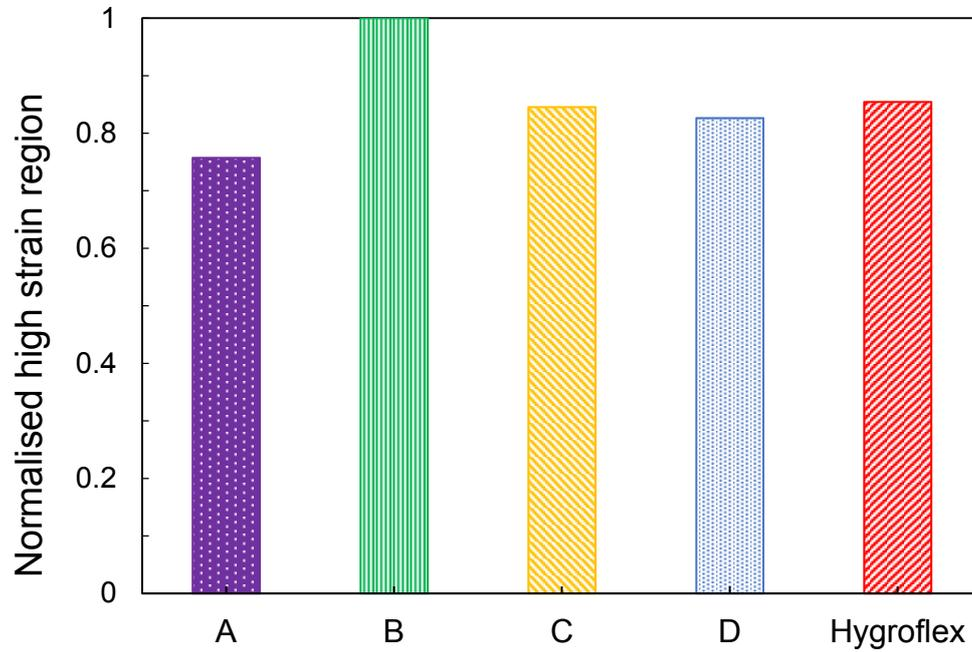
Figure 2-6: Normalised high-strain region for all foam materials under 40 % strain from sharp indenter.
