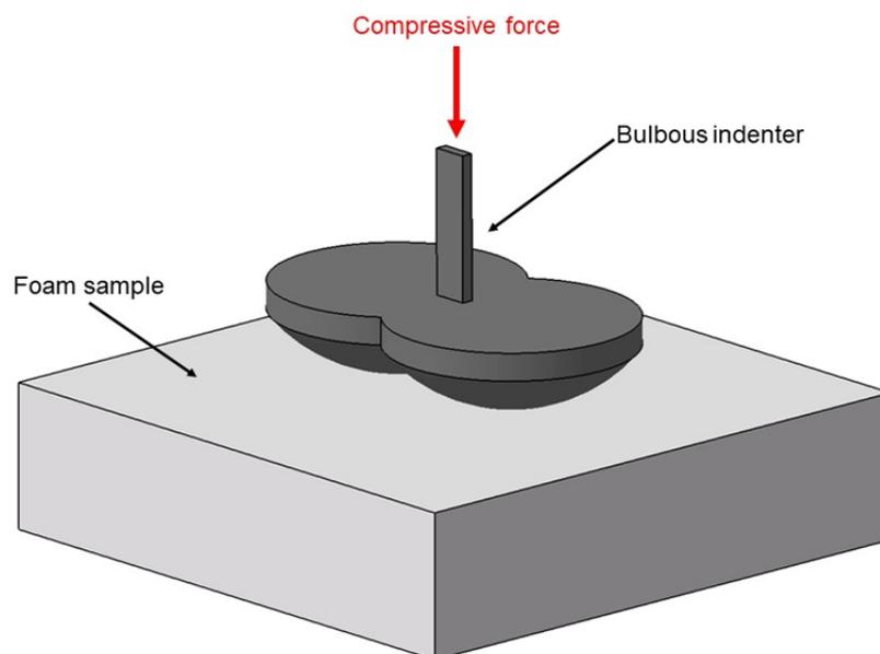
Figure 2-10: Schematic of bulbous indenter test method.
