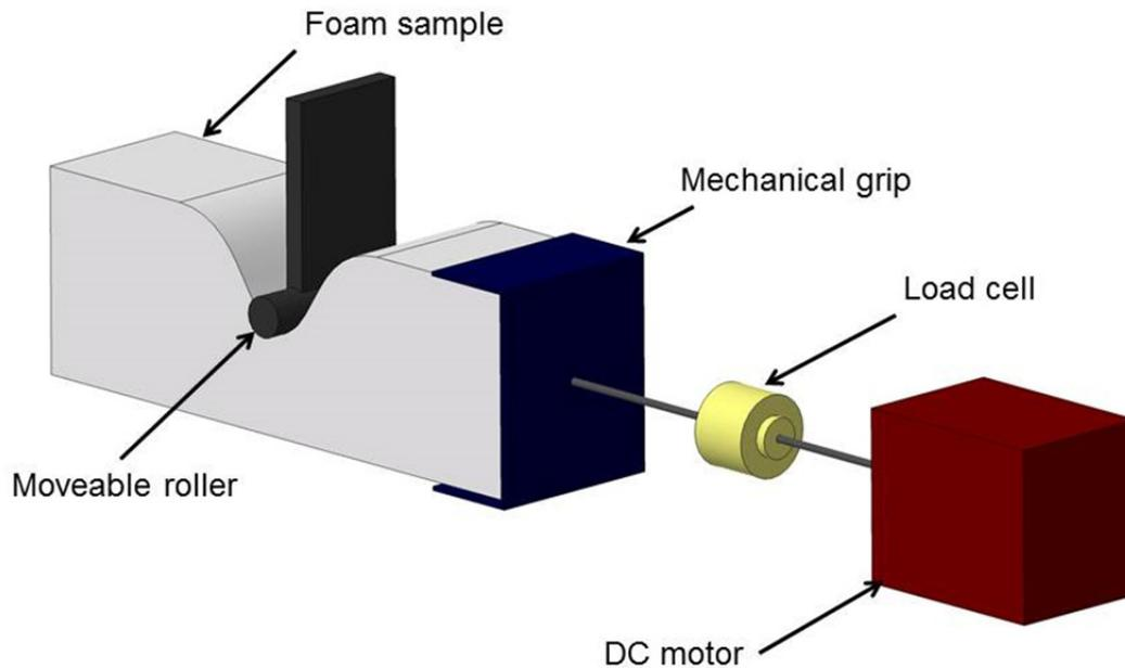
Figure 2-16: Schematic of roller-arm test method.
