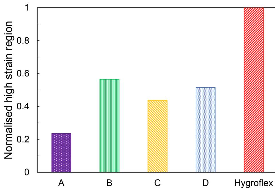
Figure 2-3: Normalised high-strain regions for all foams under an 8 N compressive force in the sharp indentation test.
