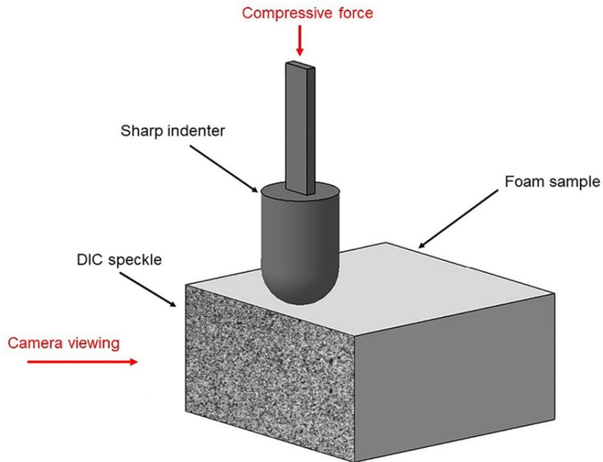
Figure 2-1: Schematic of sharp indenter test method.
