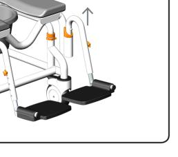
To swing the footrest out of the way sin lift the leg out of the slot and spin the leaway.
