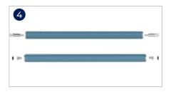
5. Place the Grab Bars in between the arms of the Upright Frame. Secure the top Grab Bar with the sling anchors bolts and the bottom Grab Bar with the two bolts as shown. Tighten and secure bolts to lock in place. Use the two plastic caps to cover the holes in the Upright Frames.
