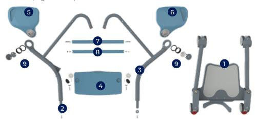
Insert each Side Frame into the base, these are notched on the end to ensure they locate correctly.
