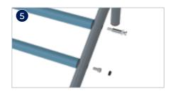
6. Fasten the Upright Frame to the Base Unit using a large washer and bolt. Tighten the bolt firmly. The bolts are provided with threadlocker on the thread, if this is missing or more is required, medium strength 243 Loctite can be applied before tightening.
