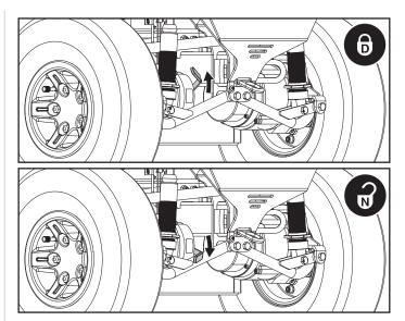
Figure 2. Manual Freewheel Lever Operation
