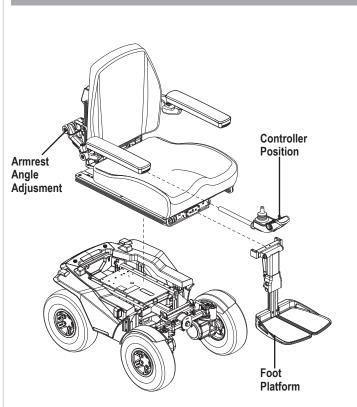
**Figure 4. Assembly View**
