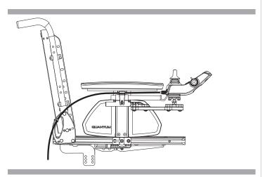
Figure 7. Controller Harness Routing on a TB-Flex Seat
