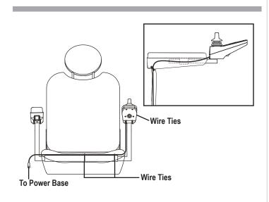
Figure 6. Controller Harness Routing on a Contour Seat
