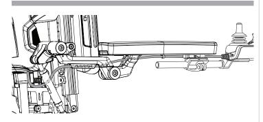
Figure 5. Controller Harness Routing on a TRU-Balance  ${\rm I\!R}$  4
