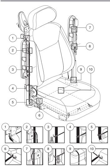
Figure 8. Controller Harness Routing on a Captain's Seat
