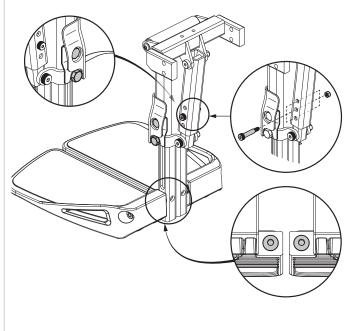
Figure 12. Foot Platform Adjustment
