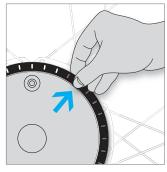
Grip the edge of the ring and press your thumbnail into the notch. Pull outwards at the same time.
