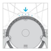
Align the new ring so that the 5 LED recesses correspond to the 5 LEDs on the drive unit.
