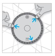
Insert the pins on the underside of the ring into the openings provided and push in the 3 locking points until they engage.
