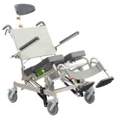
The Raz-AT600 is a heavy-duty mobile shower commode chair with a stainless steel frame and components. The specially engineered, Weight Assist Spring System (WASS) is available in two weight ranges. It is adjustable to accommodate the user's weight and Center of Mass (CoM) for tilt operation with minimal effort by the attendant.
