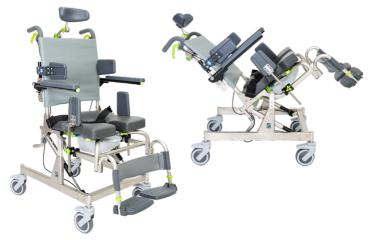
The Raz-AT mobile shower commode chair tilts up to  $40^{\circ}$  to provide extra pressure reduction and comfort. The unique frame design utilizes locking gas springs that help lift the seat to an upright position, making the Raz-AT one of the easiest tilting mobile shower chairs to operate.
